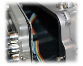
The O-ring seal is the main barrier between the water outside and the air space within the camera. It is an effective barrier only if the seal is properly maintained. The O-ring seal should be inspected before every dive. The following information is provided for guidance in using and maintaining the O-ring seal.
